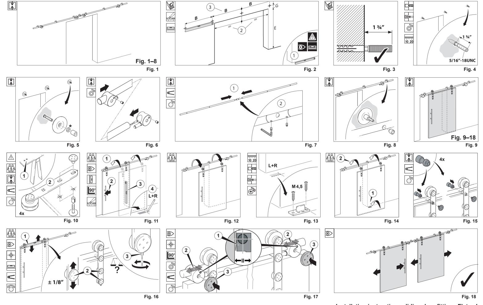
Installation instructions sliding door fittings Flatec I for 2 leaf wood doors ( max. 1-3/4" thickness)
